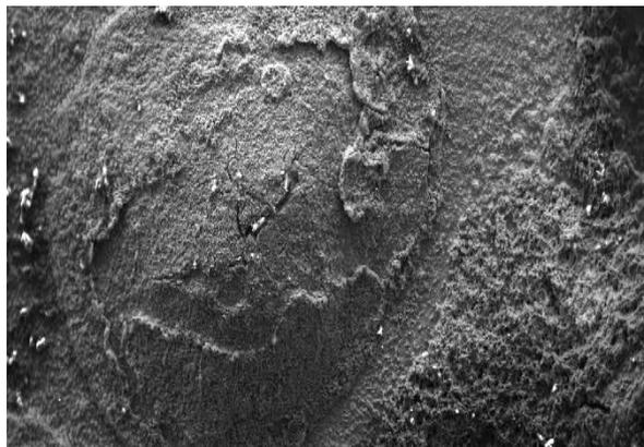
Fig. 12. Iron sulphide pitting localized attack. (500 X).
